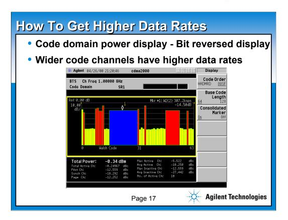
This is a "Bit-reversed" display of the Code Domain Power curve of the same cdma2000 signal. The fat blue bar in the center is the same high data rate traffic channel that occupied the many blue colored code channels on the previous slide. The total power is the area under the curve. To accomplish this simplified display, the order of the code channels on the display is altered to a "bit-reversed" order.
