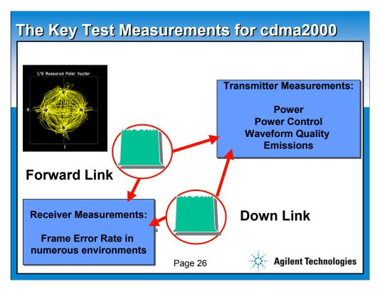
The important RF measurements for cdma2000 are shown here
