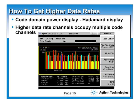
This is a display of the Code Domain Power curve of a cdma2000 system signal. Code Domain Power is an indicator of modulation quality. Using this measurement, you can verify that each Walsh channel is operating at its proper level and can quantify the inactive traffic noise level.
