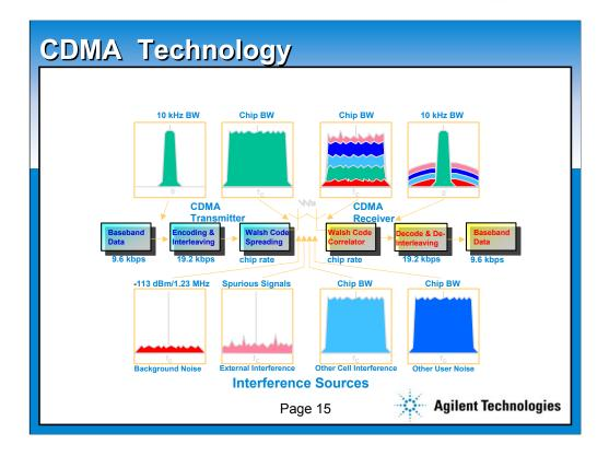
The fundamental concept of CDMA is that each user is assigned a unique code. The data for that user is spread from a low data rate (shown here as 10 kbps) to the final spreading rate, either 1.2288 or 3.84 MCPS (Mega Chips per second). Many users share the same frequency. When the de-code is applied, the proper code goes back to the 10 kHz bandwidth, while every other code stays at the full bandwidth. The portion of energy from the wide signal that falls
