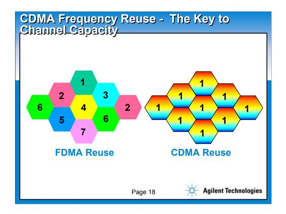
The major capacity advantage of CDMA is realized by many technical innovations. One of the most important is the reuse of the same frequency in every sector of every cell. In IS-136 and analog cellular systems, there is a 7 cell repeat factor, with 3 sectors. This means that only one out of every 21 channels is available to each sector. GSM usually uses a repeat of 4, with 3 sectors, for a reuse of one out of twelve. This is not the only factor that has
