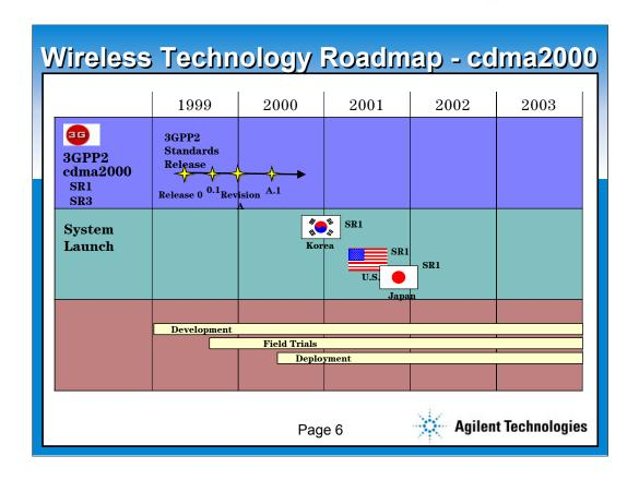
cdma2000 is going to undergo a rapid rollout. This technology is an upgrade to the existing IS-95 systems, and generally can be installed with card changes at the base stations rather than all new equipment. The conversion of handsets from IS-95 to cdma2000/IS-95 will be very quick once service starts. SK Telecom in Korea is ahead in their rollout plans, with the rest of the world showing schedules at least 1 quarter
