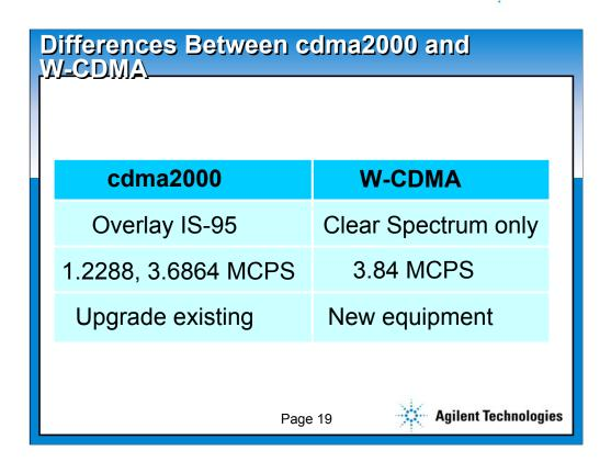
The cdma2000 system is an upgrade to IS-95. It has been designed to share the same frequency in each sector of each cell. For each user that uses cdma2000 coding rather than IS-95, the system is more efficient. Existing equipment can be upgraded to install the new technology.
